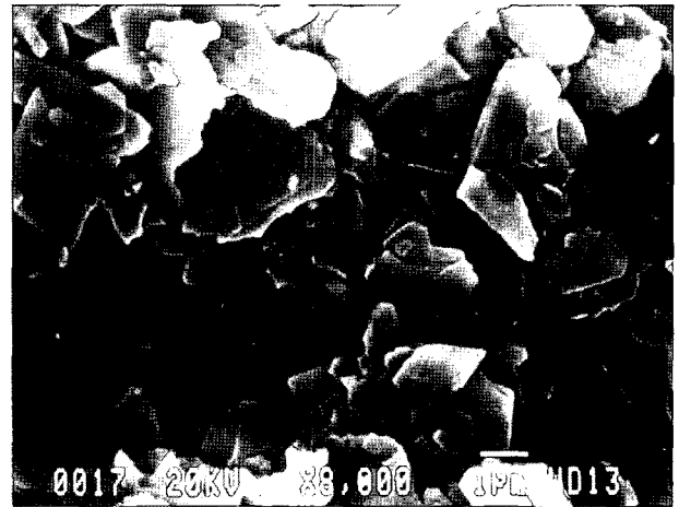
Fig. 7. SEM image of the non-swelling property mica hydrothermally synthesized at 260°C for 72 hrs in a 8M-KOH solution.
