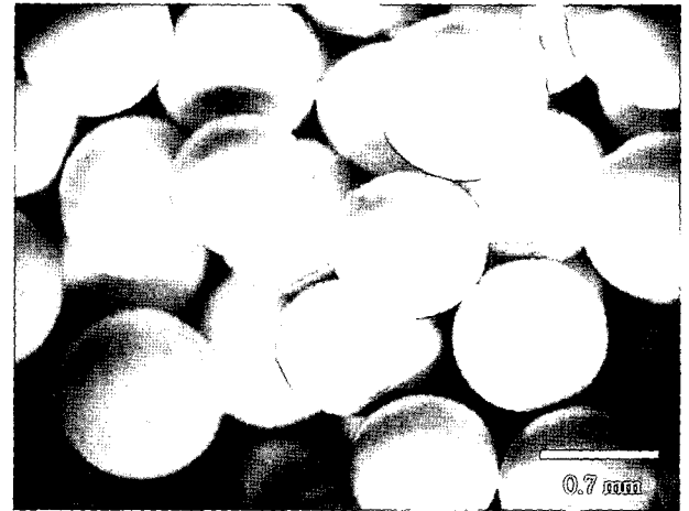
Fig. 2. Optical micrograph of zircon beads used for hydrothermal synthesis of the non-swelling property micas.
