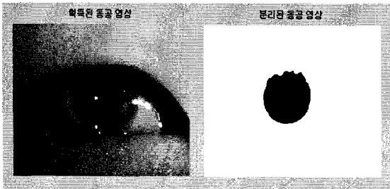
Fig 5. Binary progress for Calculation of Pupil area
