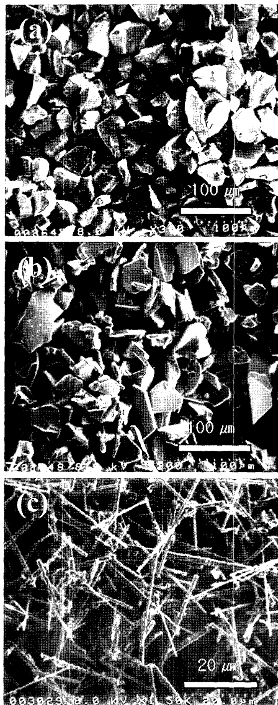
Figure 4. SEM images of silicon carbides used in this study: (a) particulate SiC; (b) platelet SiC; (c) whisker type SiC.
