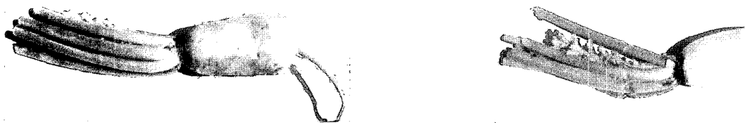
Fig. 11 Radish shapes before (left) and after (right) peeling on the rotating blade type peeling device.
