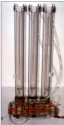
Fig. 5. An apparatus used for measurement of volume change
