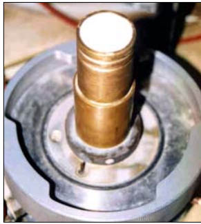
Fig. 4. Ceramics, porous disks, teflons, and O-rings used for unsaturated soil tests
