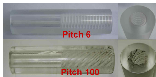
Fig. 5. Grain configuration of pitch 6 and pitch 100
