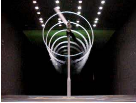
Fig. 6. The interaction of rotor tip vortices with a body (www.nrel.gov)
