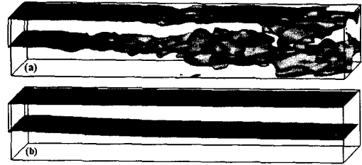
Fig. 6 Instantaneous iso-contour of streamwise velocity (6m/s) using (a) LES and (b) unsteady RANS for Re=22,100
