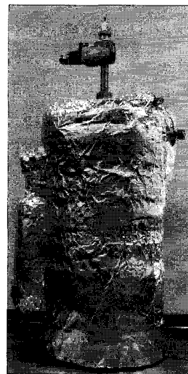
Fig. 2 Appearance of natural gas fuel processing system (height: 500 mm, diameter: 280 mm)
