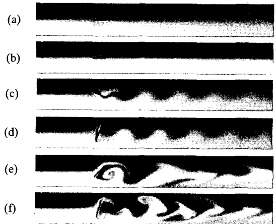
Fig. 4 Concentration distributions for various cases ; (a) Re=10, without stirring (b) Re=80, without stirring (c) Re=10, rotating, 200rpm (d) Re=10, oscillating, 200rpm (e) Re=80, rotating, 600rpm (f) Re=80, oscillating, 600rpm
