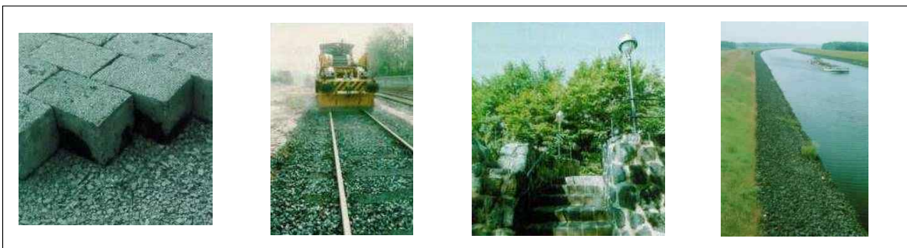
Fig. 3 Germanic copper slag practical use present condition.(Block for walk place, base materials of railroad, block for landscape architecture, Elbe River canal basin of attraction riverside construction from left)
