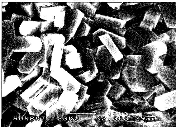
Fig. 3. Surface of ZSM-5 zeolite membrane on sintered SUS tube.
