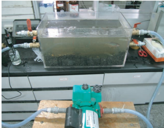
Fig. 4-a. Continuously mixed water bath for fish mortality test.
