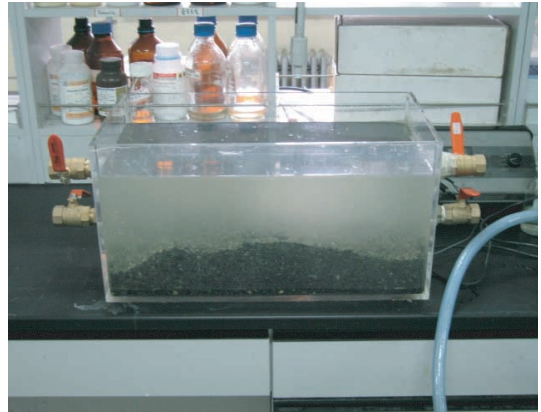
Fig. 4-b. Still water bath for fish mortality test.
