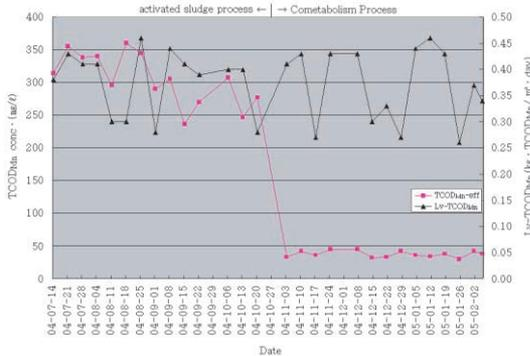
Fig. 11. Effect of TCODMn removal at different loading volume (Lv).
