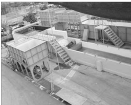
Fig. 2 Experiment flume and water supply. Fig. 3 Experiment setup of groynes for L/l=2 . Fig. 4 Measurement of velocity using ADV.
