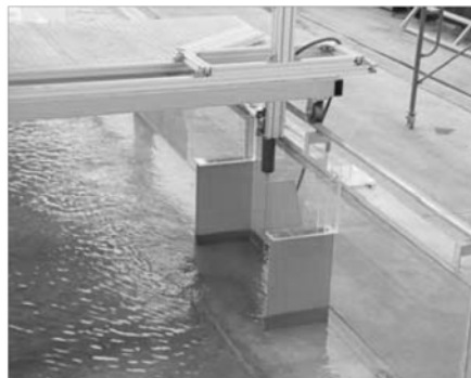
Fig. 2 Experiment flume and water supply. Fig. 3 Experiment setup of groynes for L/l=2 . Fig. 4 Measurement of velocity using ADV.
