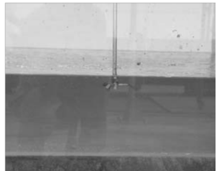
Fig. 2 Experiment flume and water supply. Fig. 3 Experiment setup of groynes for L/l=2 . Fig. 4 Measurement of velocity using ADV.
