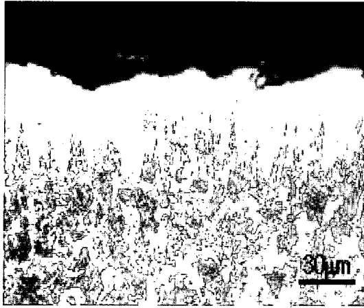
Fig. 3. Optical micrograph of the cross section of the borided AISI 1045 steel prepared by a two-step plasma boronizing process at 266 Pa in an atmosphere of 1.5 vol% BCl 3 , 50 vol% H 2 , and balance Ar. The specimen was plasma boronized for 1 h at 650°C and subsequently for 7 h at 800°C. Then, the specimen was air-cooled.
