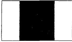
Fig. 10 The 3 rd type of the initial condition for the concentration distribution used in the simulation; horizontally separated with three regions(called HS3). c = 0 for black and c = 1 for white
