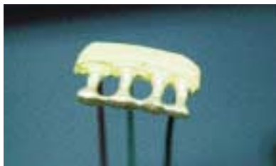
Thin, applied conductive silver lacquer with connect to the contact rod
