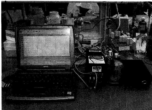
Fig. 7 Fiber-optic biosensor measurement system (from left, control computer, Analyte 2000, reagents immobilization automation block, pump controller).
