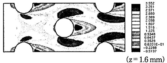
Fig. 6 Contours of U -component velocity ( Re_D = 1486 ).
