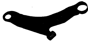
Fig. 3 Lower control arm
