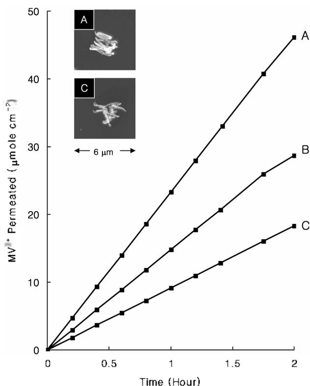
**Figure 4.** Amounts of  $MV^{2+}$  permeated through Au nanotubes prepared on solutions of  $[Au^+] = (A) 32, (B) 7.9,$  and  $(C) 4.0$  mM at  $25^\circ C$ . Insets show corresponding SEM images of nanotubes. For a SEM image corresponding to B, refer to B<sub>2</sub> of Figure 3.
