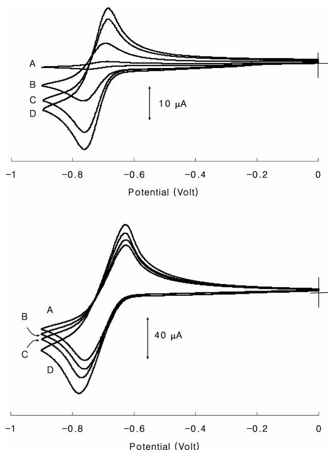
**Figure 2.** CVs of  $MV^{2+}$  diffused, from a solution containing 0.1 M  $MV^{2+}$  and 0.1 M NaCl to  $MV^{2+}$ -free NaCl solution, through Au nanotubes prepared at (A) 4, (B) 25, (C) 50, and (D) 75 °C (top) before and (bottom) after removal of a Au film on SCF. Scan rate 0.1  $Vs^{-1}$ .
