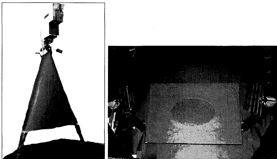
Fig. 1. Measurement condition using the GER 2600 spectrometer in laboratory.
