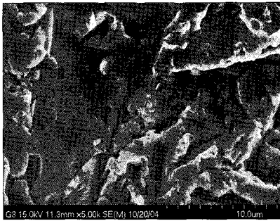
c. 250µm Sandblasted surface.
