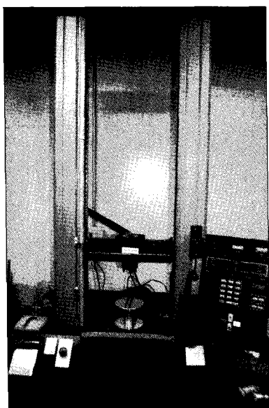
Fig. 1. Universal testing machine and shear bond test.
