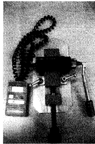
Fig. 3. 3i torque driver positioned in the digital torque gauge
