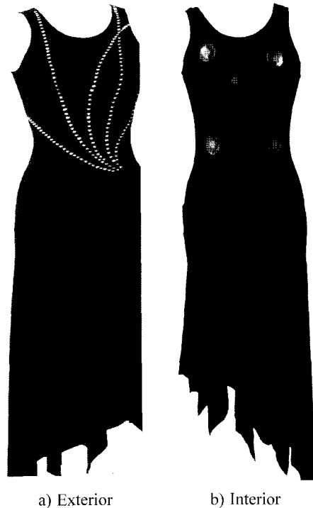
Fig. 6. Garment apparatus for measuring ECG.
