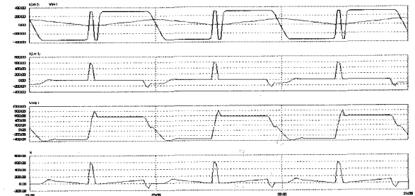
Fig. 10. Enlarged waveforms of I_{m1} , V_{ph1} , I_{rs1} , and V_{crs1} .
