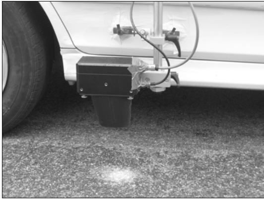
Fig. 1 Non-contact optical sensor, speedometer
