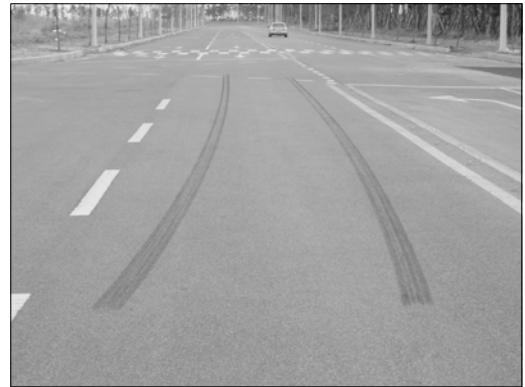
Fig. 3 Dry asphalt pavement road for vehicle test
