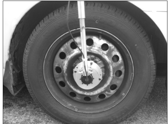
Fig. 2 Attachment of wheel rotation speed sensor
