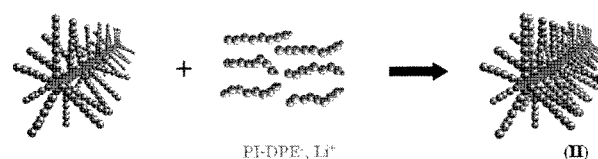
Scheme IV. Sketch for the synthesis of combs with randomly distributed PS and PI branches.
