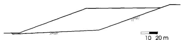
Fig. 4. Geometry of the Landfill Lying on the Gently Sloping Potential Slip Surface
