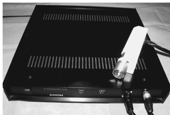
Fig. 1. The tactile sensor system(Venustron®, Axiom Co. Ltd., Japan) used for this study.
