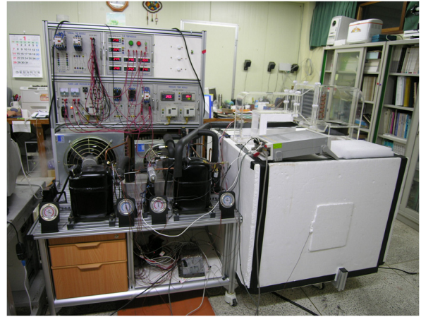
Fig. 1 Experimental device of cascade refrigeration system.
