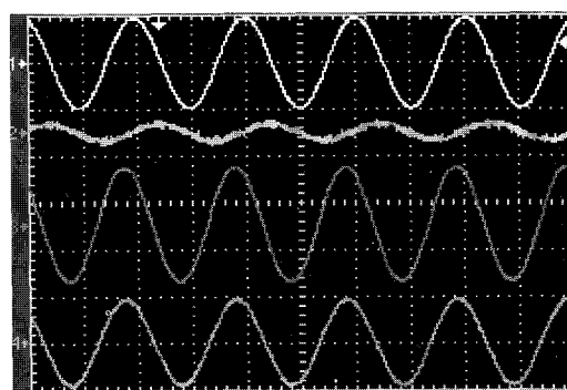
(1) AC load current -5A/div (2) Converter current -5A/div (3) IG current -5 A/div (4) IG voltage -250V/div at n = 1300 rpm
