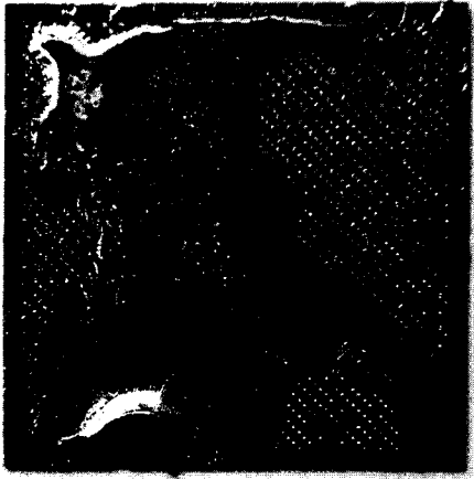
Fig. 3 Photograph showing the mold surface covered with Sn-3.0Ag-0.5Cu solder layer after ultrasonic vibration
