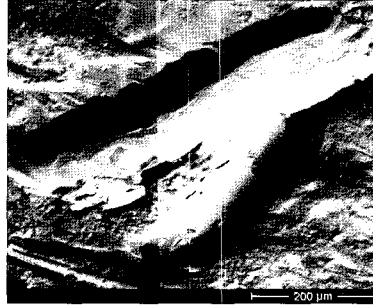
[그림 9] Influence of Impact angle on Erosion, Photograph of an Erode Surface and a Particle
