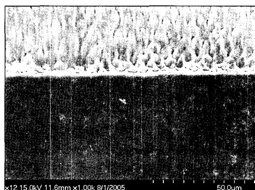
**Figure 5.** Contax and Filtek Z250 adhered to enamel.
