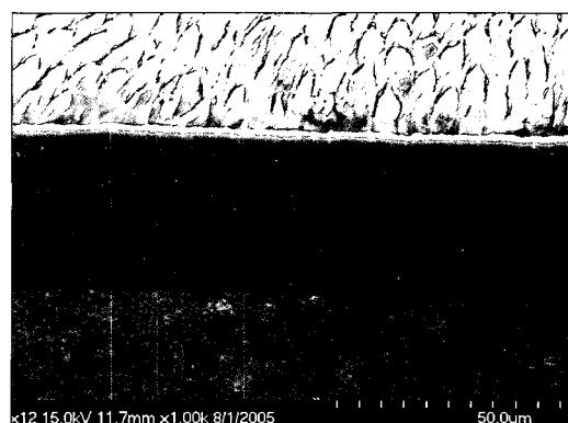
**Figure 3.** AdheSE and Filtek Z250 adhered to enamel.
