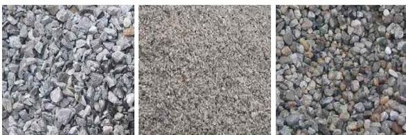
(a) Coarse aggregate (b) Fine aggregate (c) Recycled aggregate
