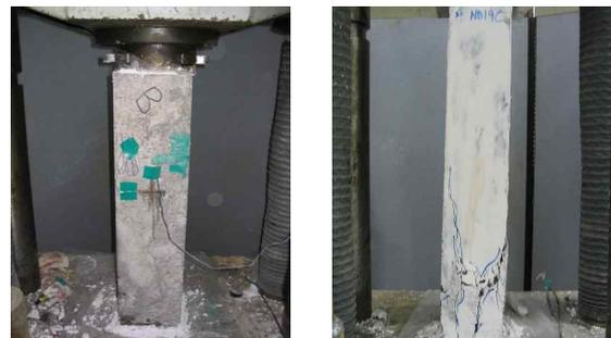
Fig. 12 Scene of recycled concrete column tests
