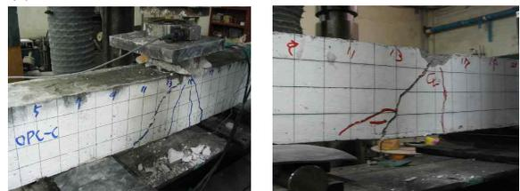
(c) Shear crack patterns
