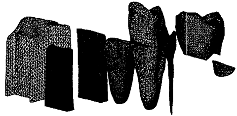
(a) (b) (c) (d) (e) (f) (g) Fig. 2 Disassembled FE model showing the different components: (a) cancellous bone, (b) cortical bone, (c) periodontal ligament, (d) dentin, (e) pulp, (f) enamel and (g) resin
