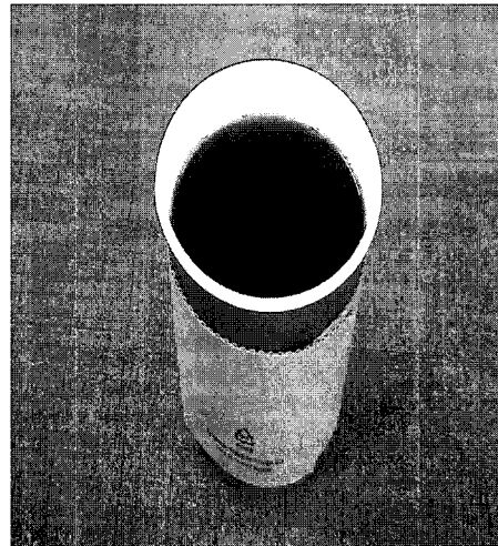
Fig. 1. Microflute paperboard packaging for wrapping hot coffee cup.
