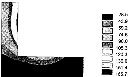
Fig. 6 Temperature distribution after heating (4 sec)
