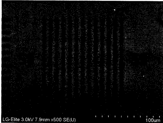
Fig. 7. PR Laser Direct Patterning Sample using Excimer Laser (L/S = 5 μm).
