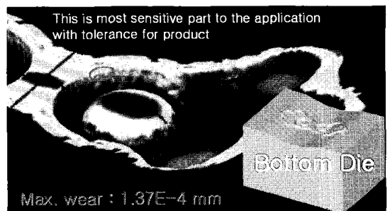
Fig.12 The most sensitive part for wear (FE simulation)
