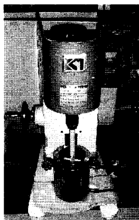
Fig. 1. Photography and dimensions of stirred ball mill experimental used.
