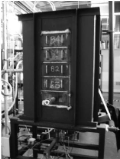
Fig. 1. MILD combustion furnace.
