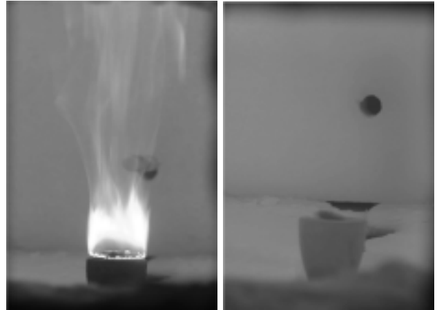
Fig. 5. Flame photo of (a) diffusion, and (b) MILD combustion of gaseous fuel.
