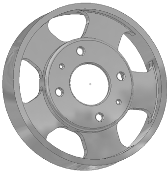
Fig. 1 3D model of circumferential pressing type brake disc
