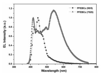
**Figure 2**. EL spectra of the EL devices with ITO/PEDOT/polymer/Ca/Al configuration.
