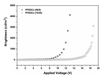
**Figure 4**. Plot of the luminescence as function of the applied voltage for the EL devices with ITO/PEDOT/polymer/Ca/Al configuration.
