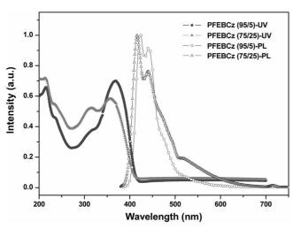
Figure 1. UV-visible absorption and PL emission spectra of the polymer films.
