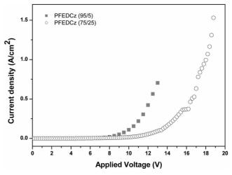
**Figure 3**. Plot of the current density as function of the applied voltage for the EL devices with ITO/PEDOT/polymer/Ca/Al configuration.
