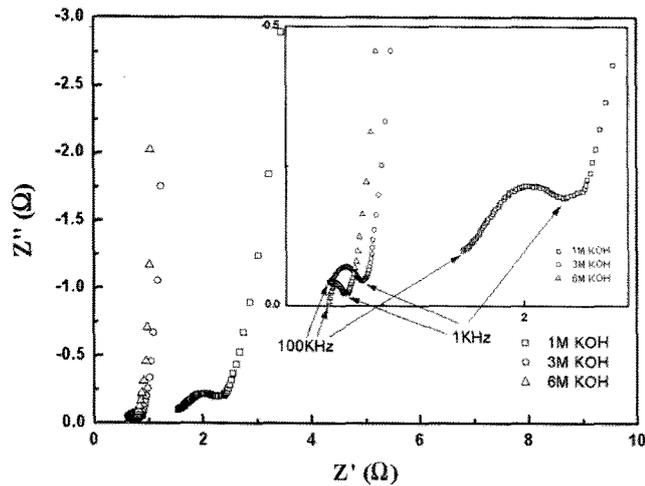
Fig. 7. Electrochemical impedance spectroscopy of carbon cryogel electrode in KOH electrolyte with different concentration.
