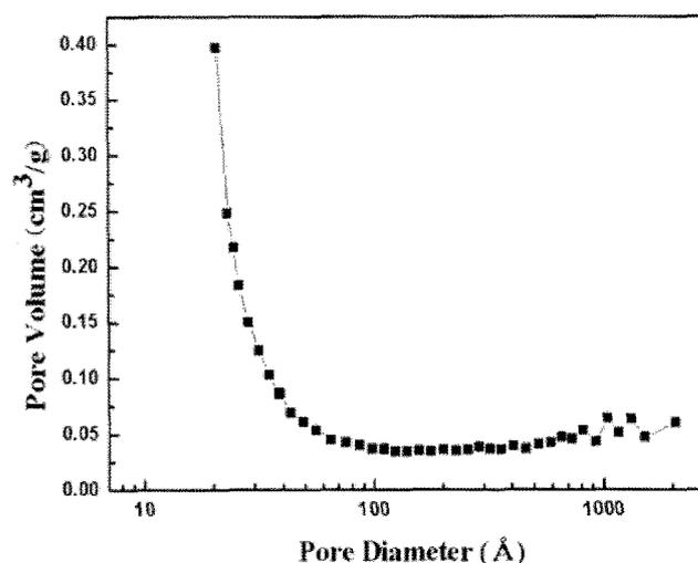
Fig. 2. Mesopore size distribution of the synthesized carbon cryogel.
