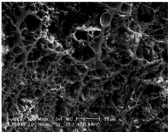
Fig. 3. SEM micrograph of the synthesized carbon cryogel.
