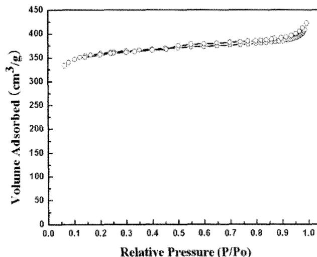
Fig. 1. Nitrogen adsorption isotherms at 77 K for the synthesized carbon cryogel.
