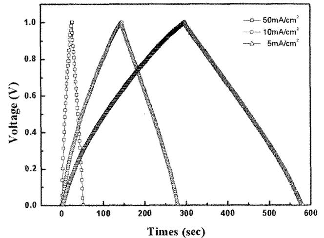
Fig. 9. Charge-discharge curves of carbon cryogel electrode measured at different current.
