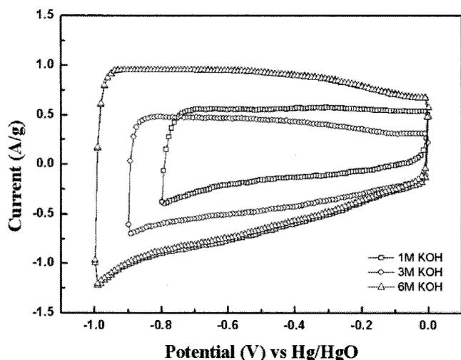
Fig. 5. Cyclic voltammograms of carbon cryogel electrode at 5 mV/s in KOH electrolyte with different concentration.
