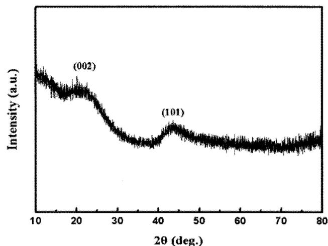
Fig. 4. XRD pattern for the synthesized carbon cryogel.
