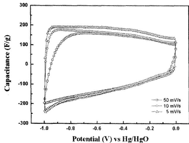
Fig. 8. Cyclic voltammograms of carbon cryogel electrode depending on the scan rate.
