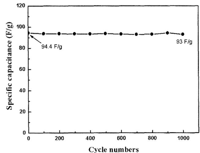
Fig. 10. Cycle life of carbon cryogel electrode measured at 10 mA/cm<sup>2</sup>.
