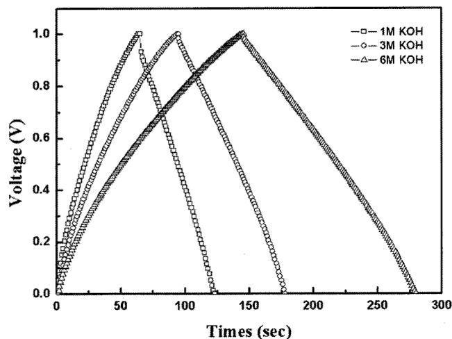
Fig. 6. Charge-discharge curves of carbon cryogel electrode at 10 mA/cm<sup>2</sup> in KOH electrolyte with different concentration.
