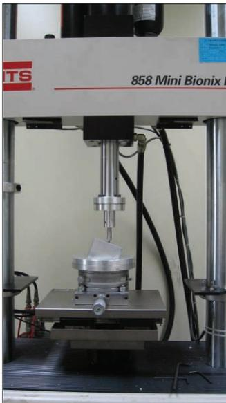
Fig. 1. Cyclic loading machine with metal jig.
