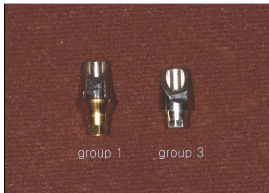
Fig. 4. Titanium abutments after preparation (group 1: internal hexagonal implant, group 3: internal octagonal implant).
